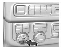
Press the Ride Height button to open the Ride Height Menu on the Instrument Panel.
