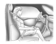
If a person of adult size is sitting in the front outboard passenger seat, but the OFF indicator is lit, it could be because that person is not sitting properly in the seat or that the child restraint locking feature is engaged. Use the following steps to allow the system to detect that person and enable the front outboard passenger frontal airbag:
