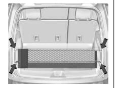
This vehicle may have a convenience net in the rear of the vehicle. Attach it to the cargo tie-downs for storing small loads.
