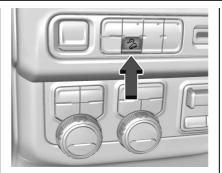
Press at to enable or disable HDC. Vehicle speed must be below 60 km/h (37 mph).
