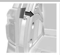
2. Remove the middle trim piece by pulling towards the center of the vehicle to disengage the clips.
