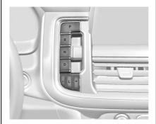
The shift switches are on the center stack. The selected gear position will illuminate red on the shift switch, while all others will be displayed in white. If the shift is not immediate, as in very cold conditions, the indicator on the shift switch may blink until it is fully engaged.
