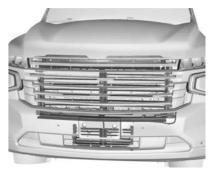
The vehicle may have a shutter system designed to help improve fuel economy. Keep the shutter system clear of debris, snow, and ice. The check engine light may activate if the shutter system is blocked.
