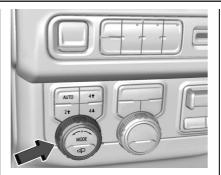
To activate each mode, turn the Mode knob on the instrument cluster to the left of the steering wheel.
