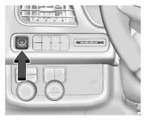
The Electric Parking Brake (EPB) can be applied when the vehicle is off. If there is not enough electrical power, the EPB cannot be applied or released. To prevent draining the battery, avoid unnecessary repeated cucles of the EPB.
