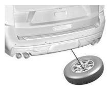
Tilt the tire toward the vehicle with some slack in the cable to access the tire/wheel retainer.
