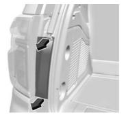
3. Remove the lower taillamp closeout cover from the taillamp assembly by pulling rearward from the top and bottom to disengage the clips.
