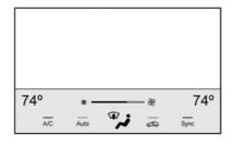
On some models, the climate control status display appears briefly when the center stack climate controls are adjusted.
