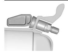
Contact your trailer service center or tire service center to have the pressure sensors installed inside the trailer tires. The technician should insert the sensor stem through the hole in the trailer wheel. When the sensor is correctly positioned, the nut on the sensor stem should be tightened to 8 N•m (6 lb ft). When mounting the trailer tire onto the trailer wheel be careful not to damage the sensor.
