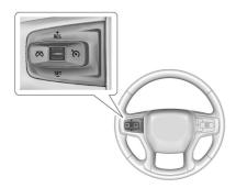
: Press to turn cruise control on or off. A white indicator comes on or off in the instrument cluster.
