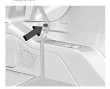
Stow the seat belt in the belt stowage clip.Repeat the steps to fold the other seatback, if desired.
