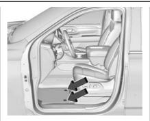
Reinstall by lining up the floor mat retainer openings over the carpet retainers and snapping into position.
