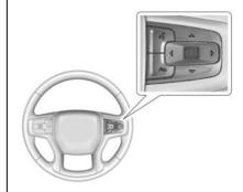
$\triangle$  or  $\nabla$ : Use the thumbwheel to scroll up or down in a list. Press the thumbwheel to open a menu or select a menu item. Press and hold to reset values on certain screens.
