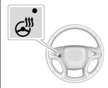
: If equipped, press to turn the heated steering wheel on or off. An indicator next to the button is lit when the feature is turned on.
