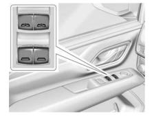
The power windows work when the ignition is on, in accessory mode, or when Retained Accessory Power (RAP) is active. See Retained Accessory Power (RAP) ⇒ 212.
