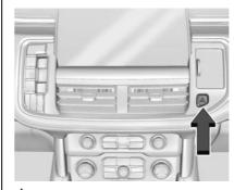
\(\triangle : Press this button to make the front and rear turn signal lamps flash on and off. Press again to turn the flashers off.
