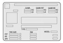
A vehicle specific Certification/Tire label is attached to the center pillar (B-pillar). The label may shows the size of the vehicle's original tires and the inflation pressures needed to obtain the gross weight capacity of the vehicle. This is called Gross Vehicle Weight Rating (GVWR). The GVWR includes the weight of the vehicle, all occupants, fuel, and cargo.
