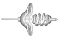
Tilt the retainer and pull it and the cable and spring through the center of the wheel.
