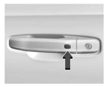
The remote key must be within 1 m (3 ft) of the liftgate or door being opened or locked. Press the button on the door handle to open. See "Keyless Access Operation" in Remote Key Operation
