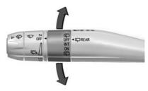
If equipped, turn the windshield wiper band fully upward or downward to spray washer fluid on the rear camera. The wipers will clear the rear camera and either stop or return to your preset speed. For more washer cycles, turn and hold the band. See Rear Camera Mirror
