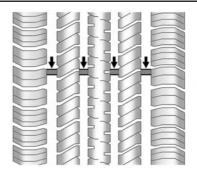
Treadwear indicators are one way to tell when it is time for new tires. Treadwear indicators appear when the tires have only 1.6 mm (1/16 in) or less of tread remaining. See *Tire Inspection* ⇔ 365 and *Tire Rotation* ⇔ 365.
