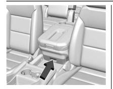
When the center console is all of the way back, there is a storage bin under the armrest. Pull on the handle to open.
