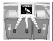
For the third row seat, the top tether anchors are on the back of the seatback. Be sure to use an anchor located directly behind the seating position where the child restraint will be placed.
