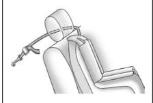
If the position you are using has a fixed headrest or head restraint and you are using a single tether, route the tether around the inboard side of the headrest or head restraint.
