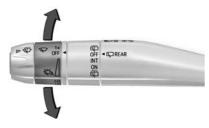
With the ignition on or in accessory mode, move the windshield wiper band to select the wiper speed.
